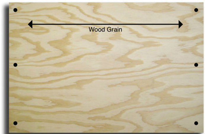
Figure 1. Plywood is strongest in the direction of its wood grain. Credits: Institute for Business & Home Safety
